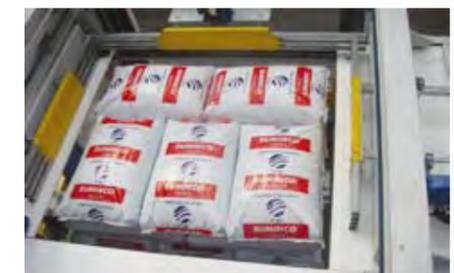
Motorized side plates for layer conforming
