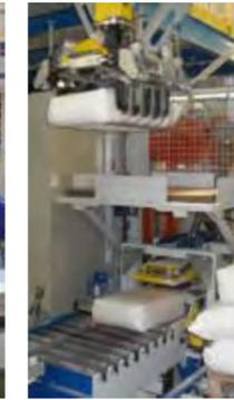
Bag conditioning by top flattening and vibrating
