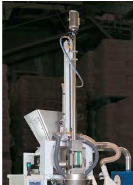
The dosing screw is easily dismantlable at the back to provide great accessibility for cleaning.
