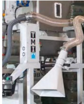
Product defluidising probe. Its function is to suck air from the product inside the bag, thereby densifying it, to allow for the immediate closure of the bag and its subsequent palletising.
